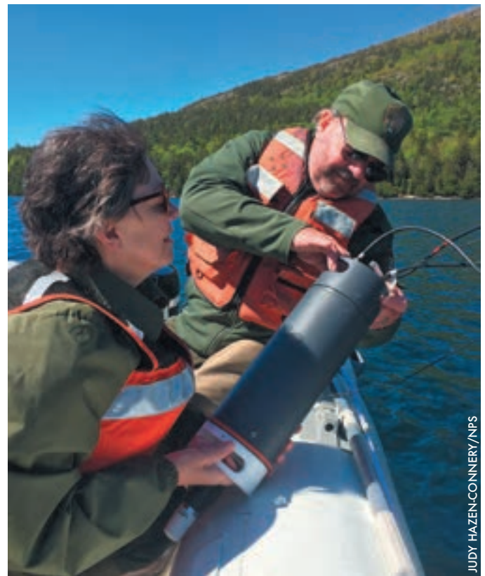
Rebecca Cole-Will and Bill Gawley install the datalogger that stores high-resolution water quality data in the Jordan Pond buoy. Below: Graphs of monthly water temperature measurements collected by Acadia National Park staff and thermal plots of Jordan Pond water temperature generated from high-resolution buoy data, recorded every 15 minutes.
